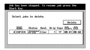
If a document is being scanned for a job, scanning stops when the [Stop] key is pressed.
